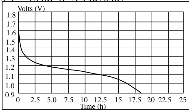
5. Load 3.9Ω ,4min./h, 8h/d, EPV 0.9V
