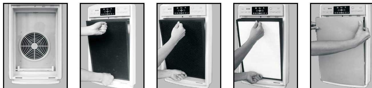
1. Open the front panel 2. Insert photocatalysator and fibre filter 3. Insert carbon filter 4. Insert the HEPA filter 5. Mount the front panel
